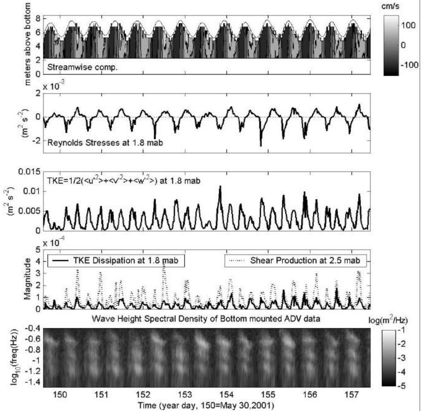
**Figure 2. Time series data from moored ADCP and ADV instruments. From top to bottom: current profiles, bottom stress at 1.8 meters above bottom (mab), the turbulent kinetic energy, turbulent kinetic energy dissipation and production rates, the sea surface wave height spectral density.**
