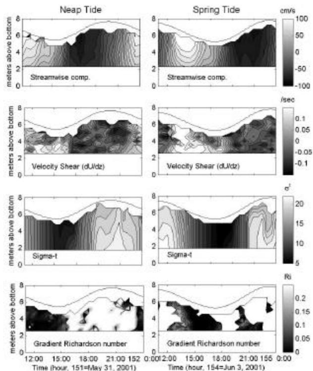
**Figure 3. Neap and spring time variations for: profiles of the along channel current speed, the density, the velocity shear and the gradient Richardson number.**
