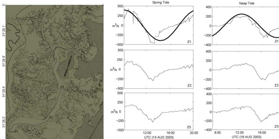
Figure 4: a) Map of the Duplin showing the location of the cross channel transects. b) Volume transport taken for each cross section in the upper Duplin River during spring (left) and neap (right) tides. Superimposed on the upper plots is the best fit M2 tidal signal.
