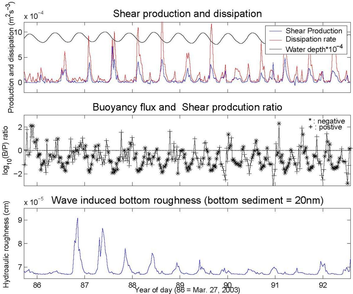
Figure 6: Turbulent kinetic energy sources in the Altamaha River estuary: shear production, buoyancy, and wave enhancement.
