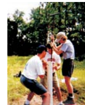
Dr. Carolyn Ruppel and GA Tech students removing the casing from a PVC hydrological monitoring well (Photo courtesy of Carolyn Ruppel)
