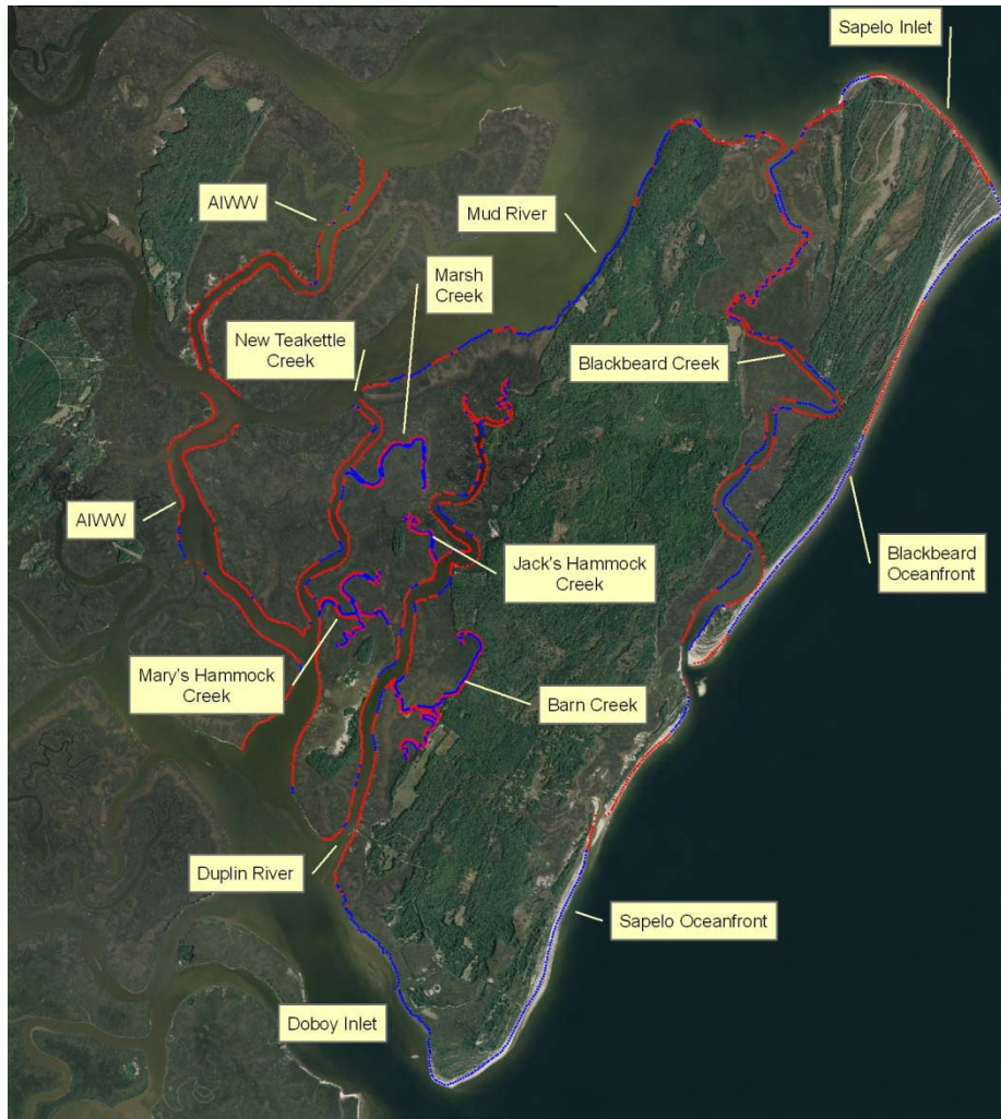
Figure 1. Areas of eroding (red) and accreting (blue) shoreline on Sapelo Island and adjacent areas. Major channels are also shown (pink), (Imagery from USGS, 2006).
